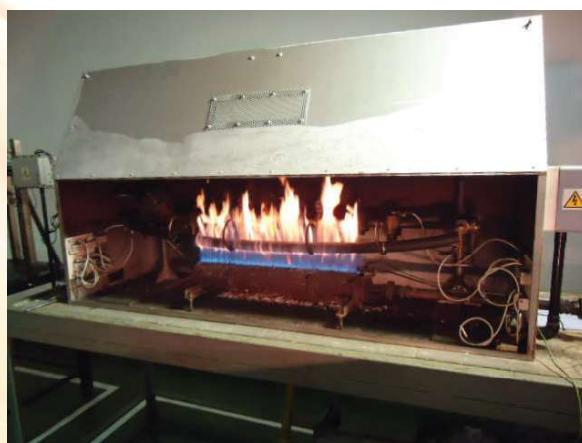
**Resistance to fire with water (Category W):** Connect the cable to the transformer same as the procedure mentioned above then attach the cable sample to the steel support then switch on the electrical supply and adjust the voltage between phases to the rated voltage. Turn on the gas supply and ignite the burner after 15 min of burning turn on the water supply. Continue the flame and water spray for the further 15 min.
